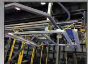
The tier sheet remover enables the Xodus™ system to remove tier sheets, inverted trays and picture frames automatically.
