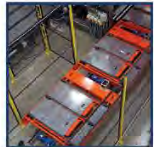
Shuttle cars mounted on a heavy duty rail system. VFD controlled bi-directional motions provide stable product movement for 2, 3, 4 or 5 pallet positions.
