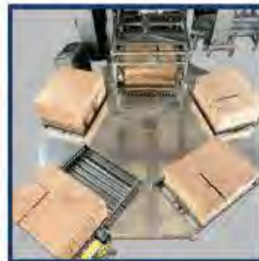
Rotary turntable is mounted on a heavy-duty cam indexer to provide smooth and rapid motion for 4, 5, 6 or 8 pallet positions.
