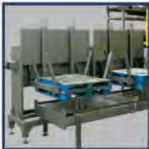
Additional pallet magazines can be added if more than one pallet size or style is to be handled.
